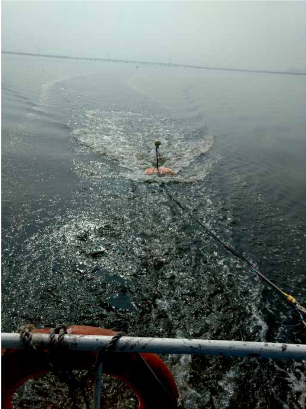
Seismic Refraction Technique Survey in progress in Thane Creek (December 2017)
