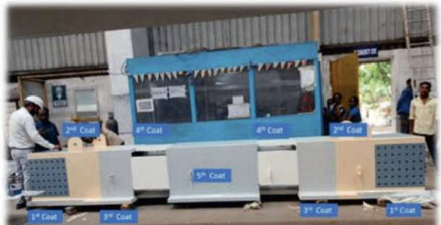
1st coat to 5th coat done on a test fabrication member for reference (out side to inside)
