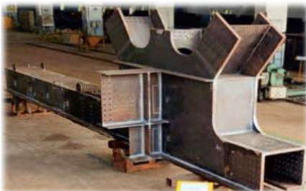
Test Fabrication of Butterfly shaped node
