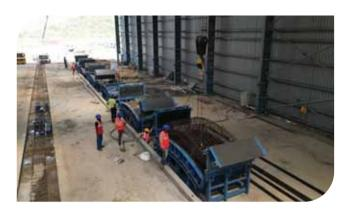
nder construction is 21 km tunnel between the Bandra Kurla Complex and Shilphata for the Mumbai-Ahmedabad Bullet Train Project. Of the total length, 16 km will be excavated using three Tunnel Boring Machines (TBMs), while the remaining 5 km will be constructed using the New Austrian Tunnelling Method (NATM). To construct the 16 km section with TBMs, 76,940 segments will be cast to form 7,441 rings. Special
