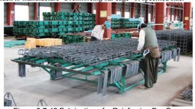
Figure 9.7-42 Fabrication of a Reinforcing Bar Cage
