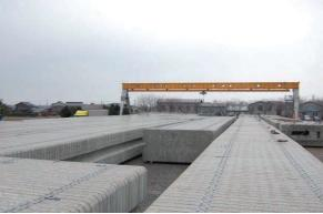
Figure 9.7-49 Wet Curing
