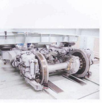
Figure 9.9-10 Bogie High-speed Rotation Test Equipment
