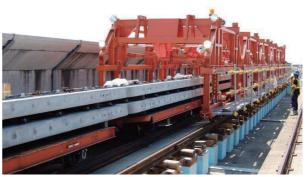
Figure 9.7-61 Lap-rail Section
