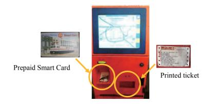
Figure 9.13-8 TVM used for the Existing Railways
