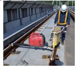
Figure 9.7-73 Measurement with a Track Master
