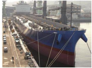
Figure 9.7-38 Long-Rail transporting Ship (Source: Sumitomo Corporation)
