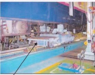
The lift of the body is carried out and a bogie is removed.
