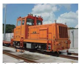
Figure 9.7-77 Rail-road Dual-mode Power Car Figure 9.7-78 Engine Power Car
