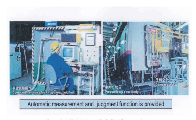
Figure 9.9-11 Airtightness Hold Test Equipment
